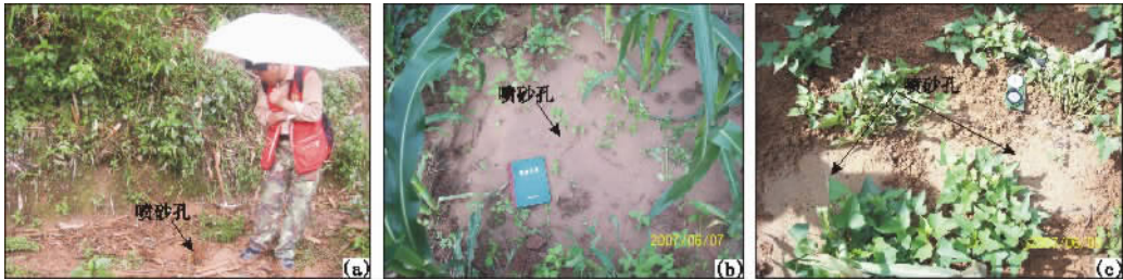
图4 宁洱地震喷砂冒水 (a) 砍柴河喷砂冒水孔；(b) 新平喷砂冒水孔；(c) 龙洞喷砂冒水孔 Fig. 4 Holes with Sandboils and waterspouts after Ning'er earthquake (a) Kanchahe hole; (b) Xinping hole; (c) Longdong, two holes
