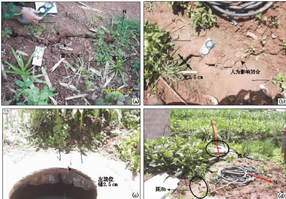
图5 北东东向地震地裂缝. (a) 新平地裂缝；(b)，(c)，(d) 昆鹅地裂缝 Fig. 5 Ground fissures of ENE-strike induced by Ning'er earthquake (a) Xinping ground fracture; (b, c, d) Kun'e ground fracture
